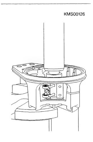
Checking commutator end shield
